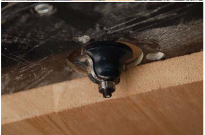
**2.** When using a router you must make sure your project is very tightly clamped in place or it will vibrate and shoot across the room.
